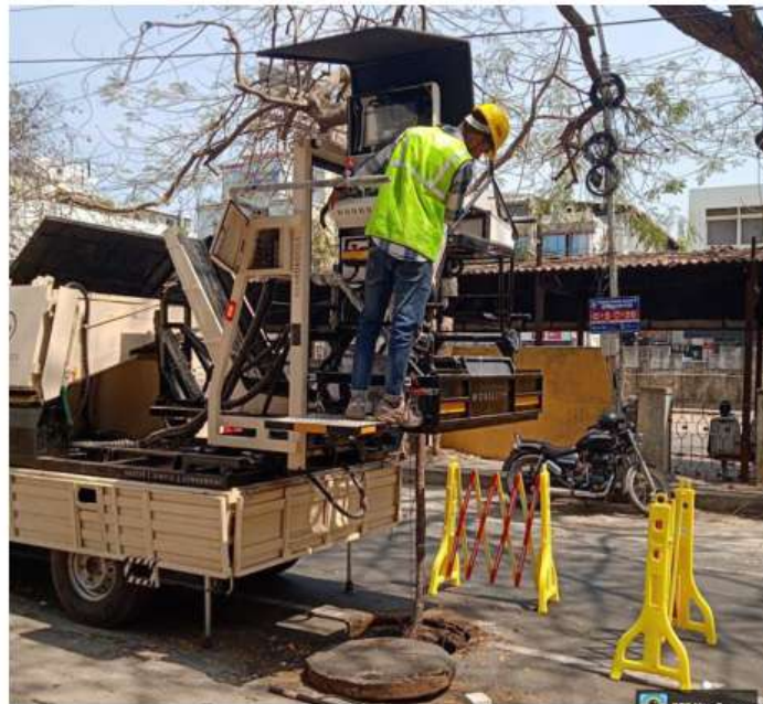
Hands-free: The device mounted on a vehicle comprises a stand unit with control panels and a robotic drone system with spider-like legs that is lowered into manholes to remove waste.
