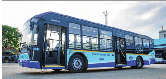
MAKING STRIDES: An e-bus can run up to 200km on a two-hour charge
