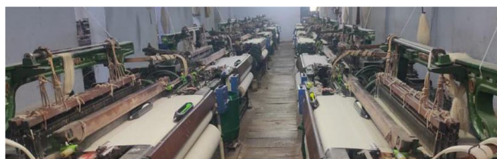
Reducing risks: The study recommends replacing the conventional looms with shuttle-less looms and installing soundproof barriers made of transparent materials on doors and windows to reduce ambient noise at a distance of 6 metres to 7.5 metres from the loom.
